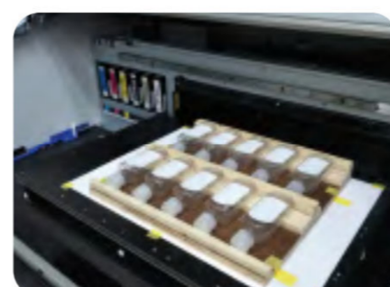
Step 1: Print white color as the first layer to enhance the vibrancy of the colors of the design
